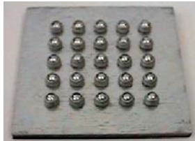
Carrier plate with 25 rivets belonging to the same batch
