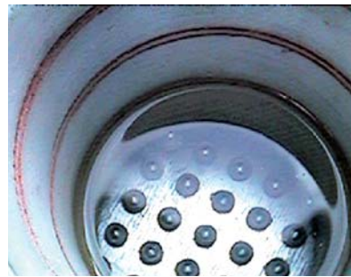
Testing the watertightness on the closing head side under 30 mm water column during 60 minutes
